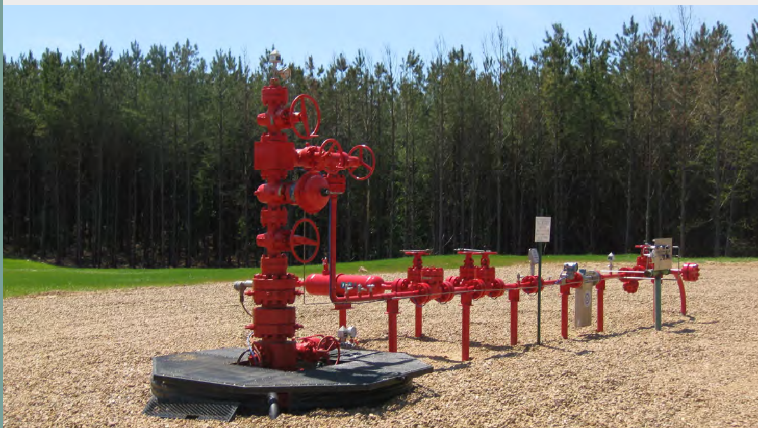
A carbon dioxide (CO 2 ) injection well drilled by the Southeast Regional Carbon Sequestration Partnership (sponsored by the U.S. Department of Energy) at the Cranfield CO 2 test site in Mississippi. Source: Geology, Energy & Minerals Science Center, United States Geological Survey. https://www.usgs.gov/media/images/co2-injection-well-mississippi . 2010.
